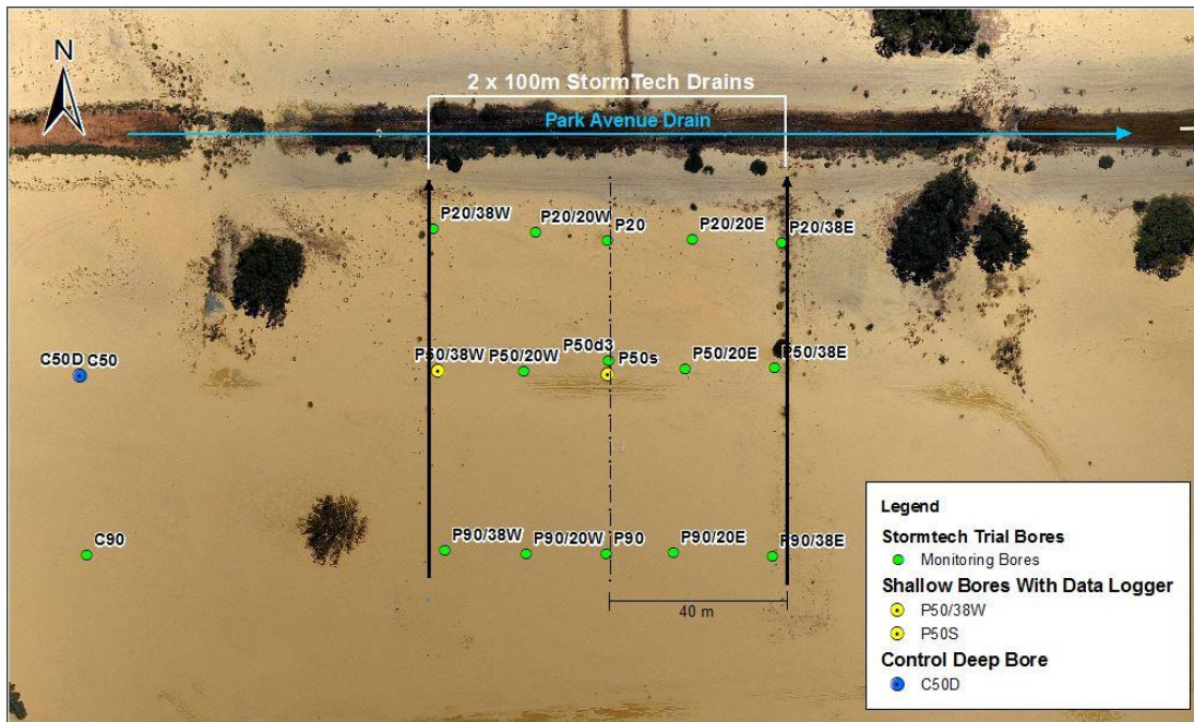
Figure 2: Monitoring Bores and Layout
