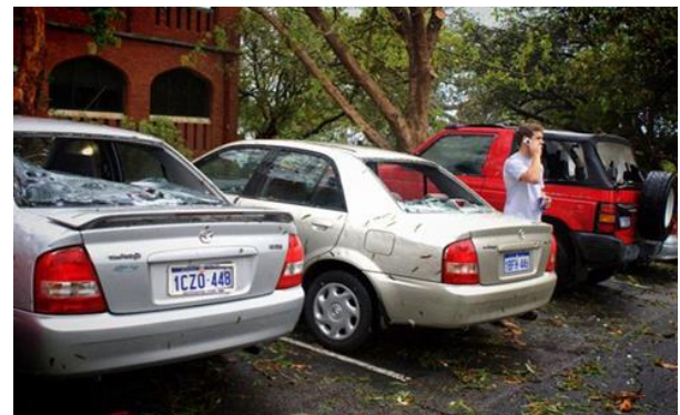
Figure 6: Hail damaged car (north-facing windows broken with significant denting) at UWA (Jarrad Seng, 2010)
