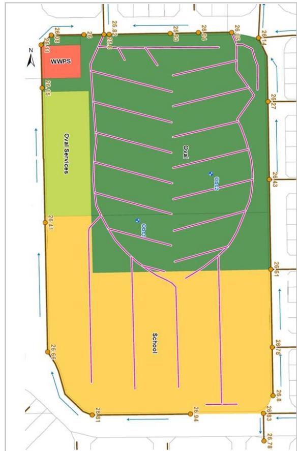
Figure 7: Subsoil Drainage Layout
