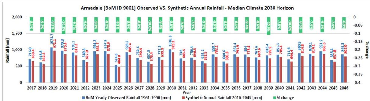
**Figure 2: Armadale Rainfall Station Synthetic 30 year Record for Median Climate 2030 Horizon**
