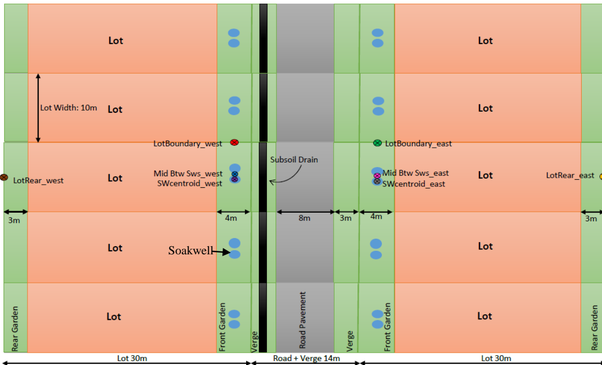
Figure 2: Soakwell (SW) 2x1.5m Diameter 1.2m Deep at the front of the Lots
